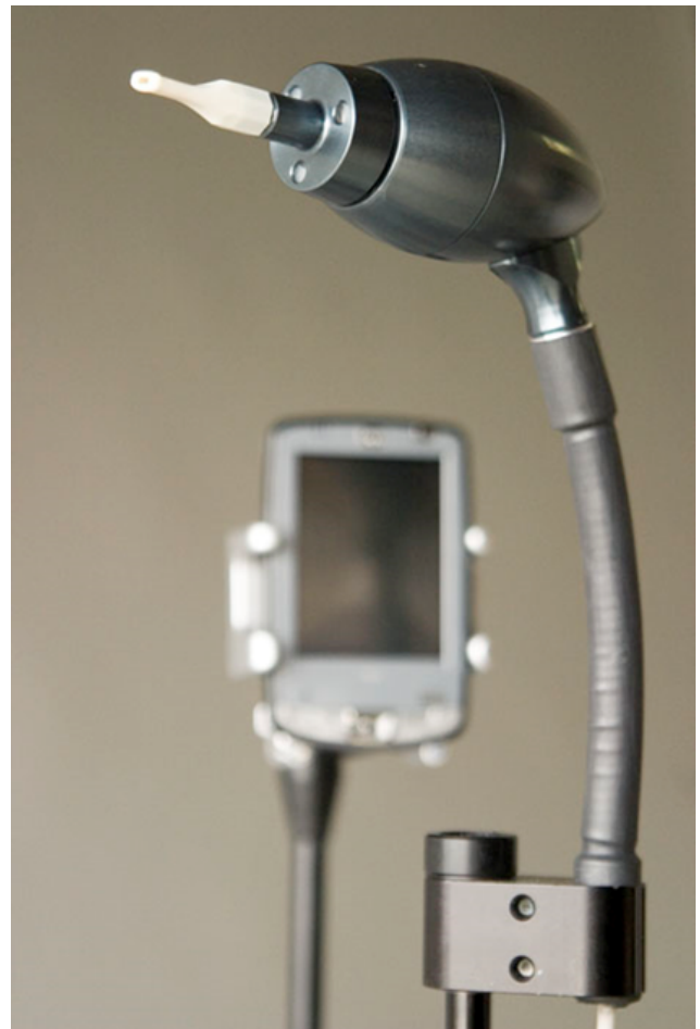
The LipSync Prototype – As of right now, the LipSync connects via specialized USB cable, however, Bluetooth support is currently being researched.
